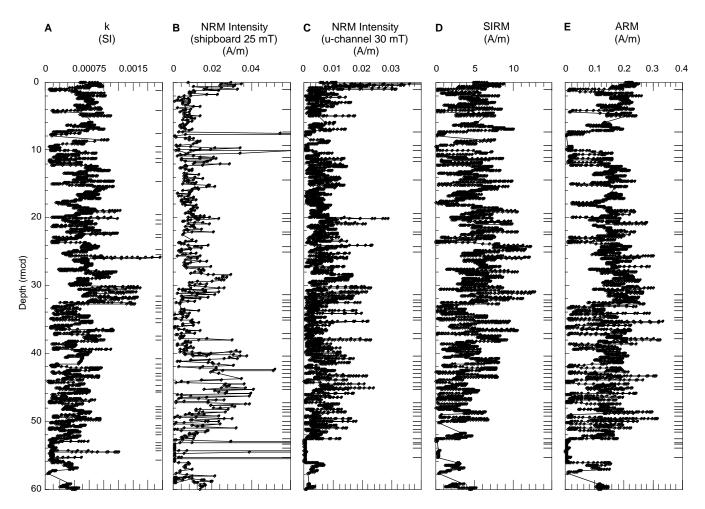
Figure 2. Shipboard and u-channel magnetic measurements from the composite sequence for Site 967 for the interval from 0 to 60 rmcd. Panels (A–E) are the same as for Figure 1.
