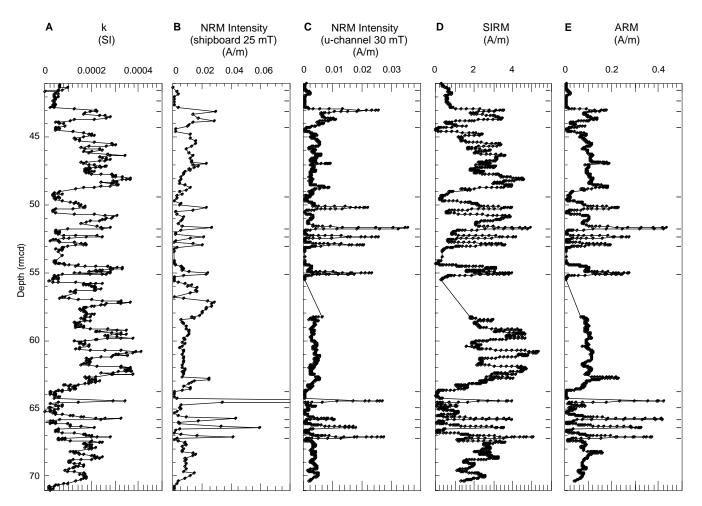
Figure 3. Shipboard and u-channel magnetic measurements for Hole 969B for the interval from ~41 to 71 rmcd. Panels (A-E) are the same as for Figure 1.
